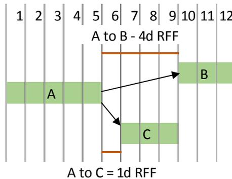
Figure 4: Relationship Free Float for an activity with two non-driving successor relationships.
