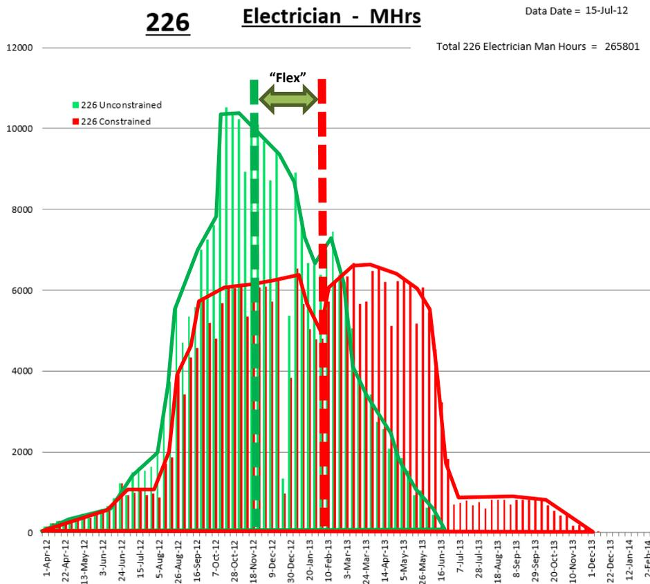
Figure 9: Electrician weekly labor hours from an update of a metal refinery project.
